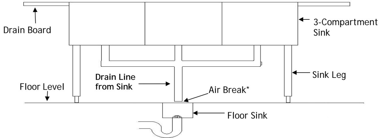
Illustration 2: Indirect drainage to three bell reducers.
