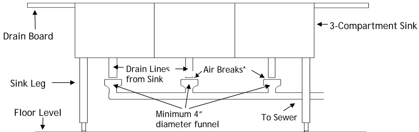
**Illustration 3:** Indirect drainage to one bell reducer.
