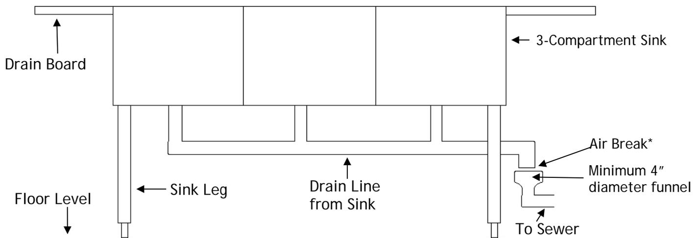
\*An air break is an interruption in the pipe that prevents sewage from flowing backwards into a sink basin or appliance.
